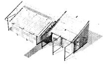
Fig. 6:. Solar PV panels on metal roofing deck with Hardie board over Structural Insulated Panels for wall infill.
